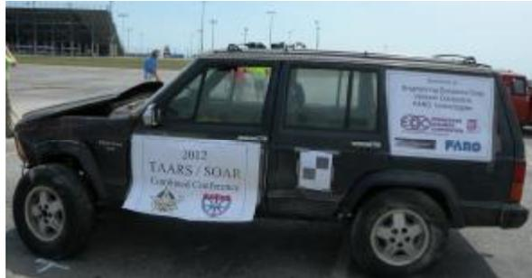
The first crash was an angular (T-bone type) crash with an older Jeep Cherokee as the bullet vehicle and a small Ford pickup target vehicle towing a single axle utility trailer with a load of concrete mix. (Note to self...never use dry concrete mix as a load in an open trailer again.) Impact speeds at 43 mph. (Note to Jeremy....be careful where you put the cameras :-)
